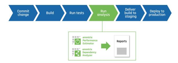
An additional 'run analysis' pass can be added after the build step. Compilable source code is a prerequisite for analysis in both tools.
