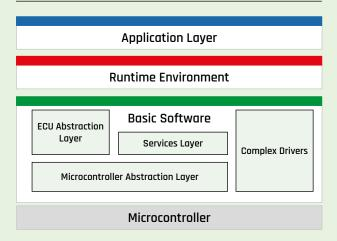
The emmtrix analysis tools ePE and eDA are designed to analyze C code on the Application Layer in the form of runnables that are part of Application Software Components (SWCs) and make up the functional part of applications. They can be considered as running isolated from the rest of the system as all interaction with other runnables is handled through function calls to the RTE.
