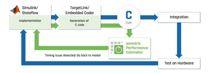
Addressing timing issues in this way is expensive and time-consuming, as the issues are detected only after integration and measurements. Manually mapping these results back to Simulink is complicated as the granularity of the information is on the level of runnables or software components as specified in AUTOSAR and not on the actual model.
